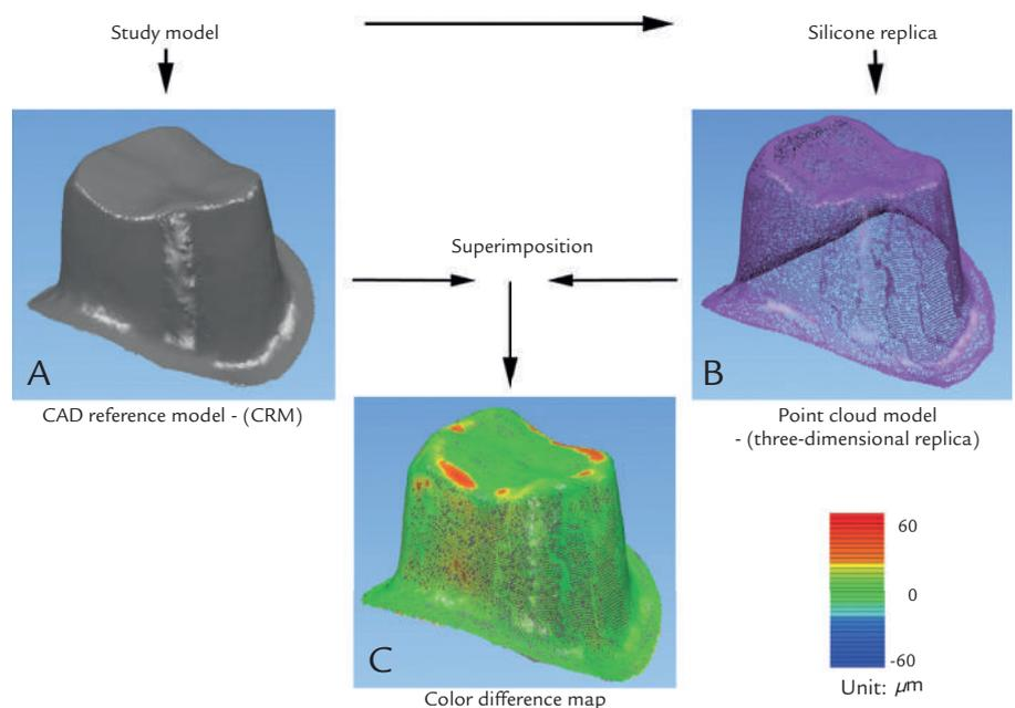
**2** Three-dimensional measurement for gap. A, Computed-aided design reference cast: digital cast by scanning stone cast with dental scanner. B, Point cloud model: model with point cloud data from digital replica. C, Color difference map: discrepancy of each point of models B and A presented in different colors.
