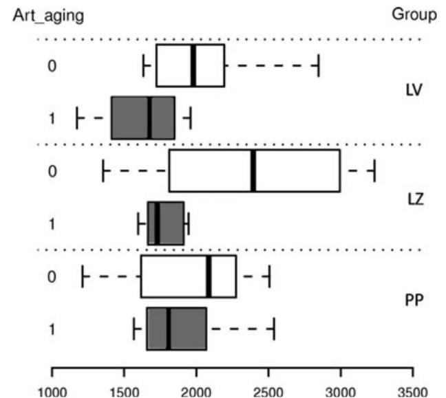
**Fig. 3.** Box plots of results of the load-to-fracture test of different groups in Newton (group LV, layering technique/Vintage ZR; group LZ, layering technique/ZIROX; Group PP, CAD/CAM and press-over techniques/PressXZr) before and after ageing (0, non-aged groups; 1, aged groups) (*n* = 8).
